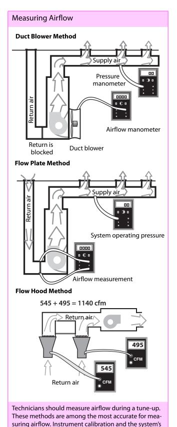
air leakage can affect testing accuracy.
