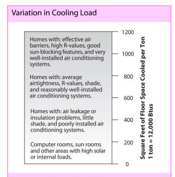
The number of square feet of floor space that can be cooled by a ton of air conditioning depends on climate, shade, insulation levels, and air leakage.
