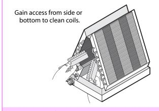
Access the a-coil from the side or underneath in upflow systems. Clean the fins by brushing, then spraying with cleanser and rinse water, if necessary.
