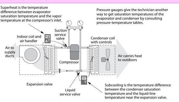
Technicians measure superheat or subcooling temperatures during summer cooling. These measurements indicate whether or not the refrigerant charge is correct.
